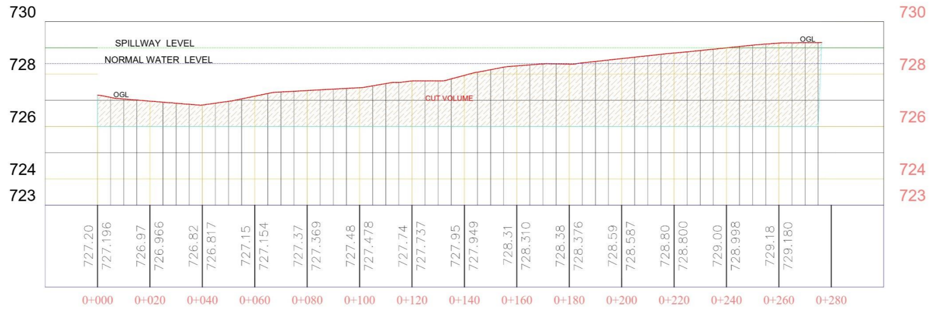
Alignment - RESERVOIR LONGITUDINAL-SECTION PROFILE
