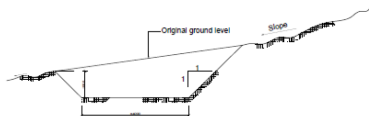
CROSS-SECTION C-C (PROTECTIVE TRENCH)
